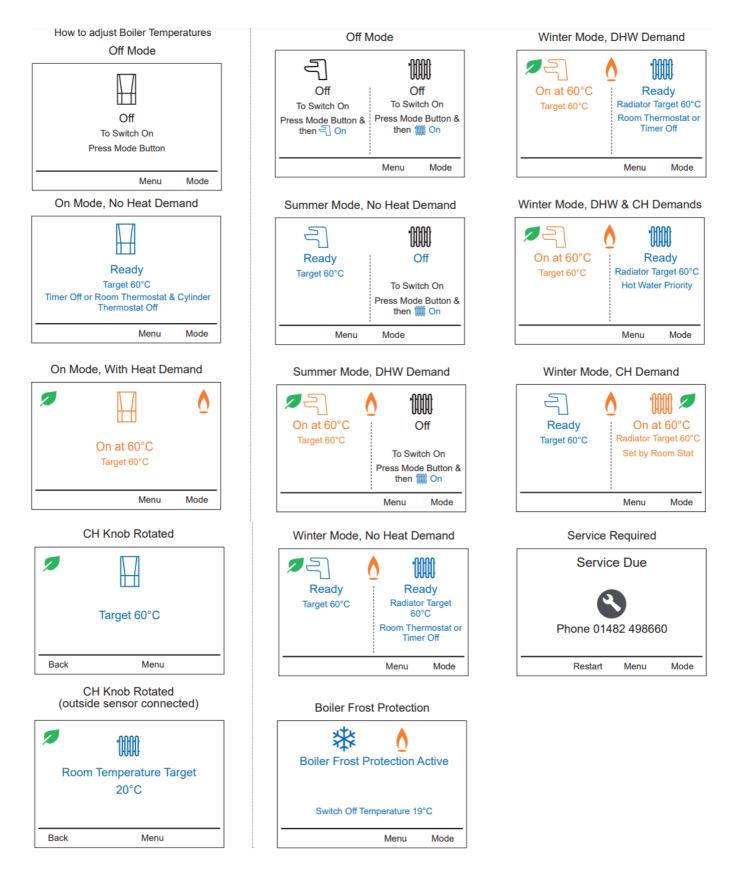
The display scrolls through a maximum of 3 messages under any operational condition, as shown above
