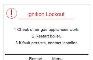
• To restart the boiler, press Restart. The boiler will repeat the ignition sequence. If the boiler still fails to light consult a Registered Gas Installer.
