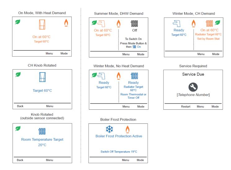
The display scrolls through a maximum of 3 messages under any operational condition, as shown above
