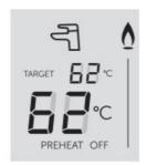
Boiler is heating up the Plate Heat Exchanger
