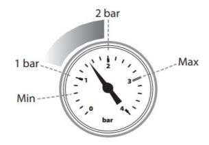
THE BOILER WILL NOT OPERATE IF THE PRESSURE HAS REDUCED TO LESS THAN 0.3 BAR UNDER THIS CONDITION.
