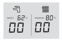
Boiler is active for Central Heating
