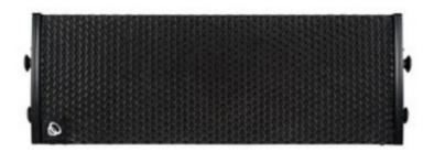
forward active system that optimises costs, setup and logistics. The HF assembly mounts a 3" compression driver and an **IDEA** proprietary Hi-Q waveguide allowing for minimum vertical gap between array elements providing optimum element coupling and reducing artifacts and DSP adjustments while providing optimum directivity control. For LMF section, **EVO**88 elements mount dual very high-performance 8" woofers.
