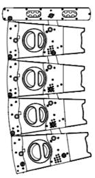
5. Elevate the four top elements to a level where the next EVO20-M elements in the transport cart naturally allaign
