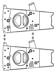
3. Finally lock the desired position with the dedicated pin stored in the Groundstack/Stow hole. Repeat the operation for the any other EVO20-M element in the system.
