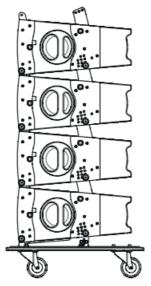
2. If the EVO20-M rigging frame structure is not already linked, proceed to lock the four rigging points of the frame to the integrated rigging structure of the top EVO20-M element.
