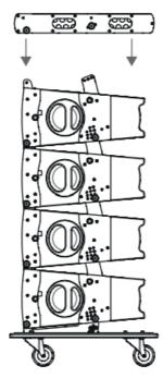
3. Unlock the bottom EVO20-M element from the transport cart and proceed to suspend the system up to a comfortable position for next step.
