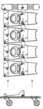
4. Set internal splay angulation according the desired setup
