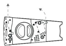
2. Position and lock the front and backlinks of the following element in the array using the spare pins stored in the dedicated hole labelled as Stow.
