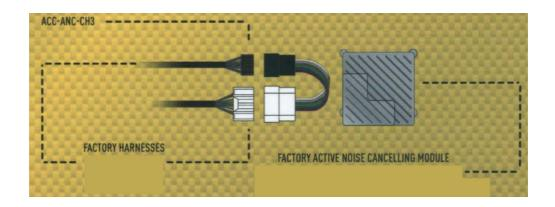
BYPASSES THE FACTORY NOISE CANCELLATION WHEN REPLACING THE RADIO OR AMPLIFIER
