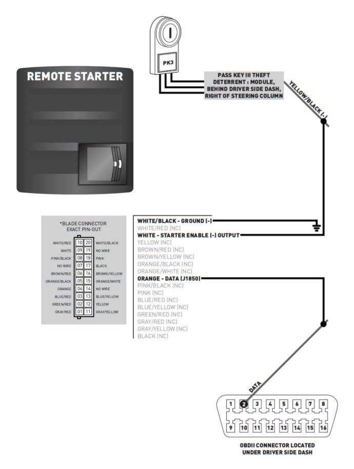
**TYPE 3 – WIRING DIAGRAM**
