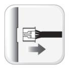
3. PRESS AND HOLD programming button while connecting the BLACK 4-PIN connector.
