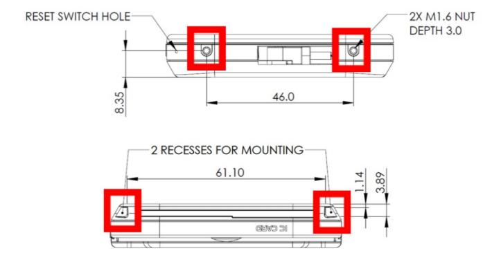
Likewise, the VP3350 has slots on the back for alignment, shown bel
