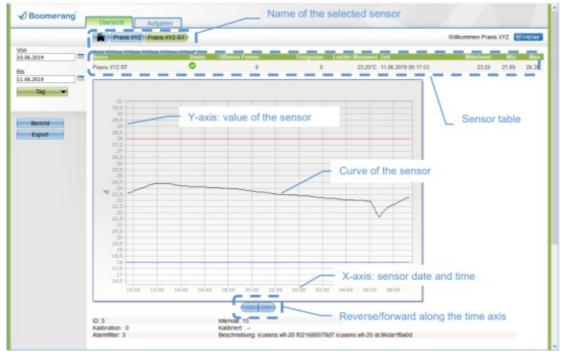
Below the diagram, the sensor ID, measuring interval, calibration value and time, alarm filter and sensor description are displayed.
