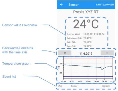
The event list is displayed below the sensor graph. In the example shown below two events are listed on 11.06.2019. The first, with a time stamp of 08:49:15, was signed by the user with the name "manual". The second, with a time stamp of 09:20:15, has not yet been signed.
