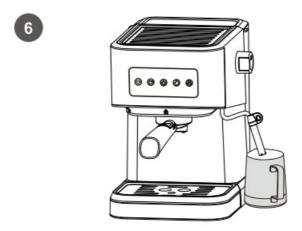
Immediately refill the water tank with clean water and repeat the process to flush the system.
