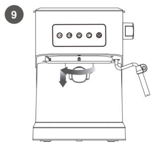
then pour coffee residue out with steel mesh pressed by funnel holder clip.
