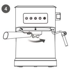
and fix them into coffee maker firmly by turn it anticlockwise until it is at the "  $\widehat{\mbox{\it l}}$  " position.
