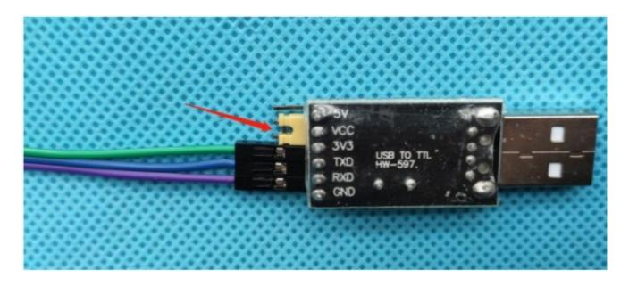
Connect the other side of the Dupont line to the download connector of the cube. The TXD of the downloader is connected to the TXD of the cube, the RXD of the downloader is connected to the RXD of the cube, and the GND of the downloader is connected to the GND of the cube.
