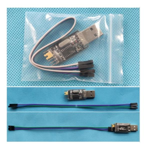
Connect the three Dupont cables to TXD RXD GND of the downloader. The yellow short-circuit cap pointed by the arrow is connected to VCC and 3V3.
