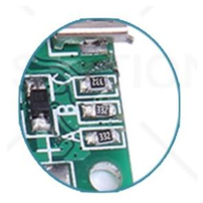
You can change to other mode by removing the resistor on the board. For example, if you want to set 001 (Under this mode, you need to hold down the button to play the music. It will stop once you release the button.), you need to remove the third resistor that marked C on the board. To remove the resistor, you need a soldering iron to melt the solder and take the resistor away. It is a little difficult if you are not good at soldering so we recommend you to use 000 default mode.
