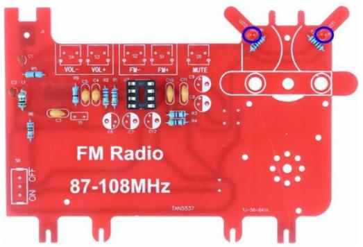
• Step 18: Install 1pcs 1P2T Toggle Switch at S6.
