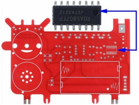
• Step 2: Randomly choose a pad on the PCB, and then melt the solder on this pad.
