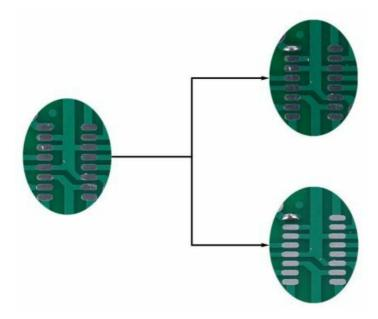
• Step 1: Melt a small amount of solder on the pad which IC can placed(It is used for positioning the chip in the next step).
