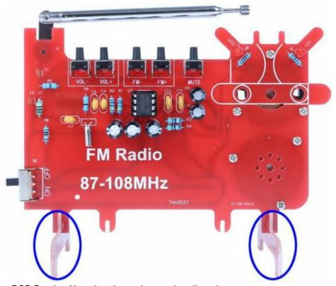
• Step 29: Fix 2pcs PCB Bracket.Note that the pads must be aligned.
