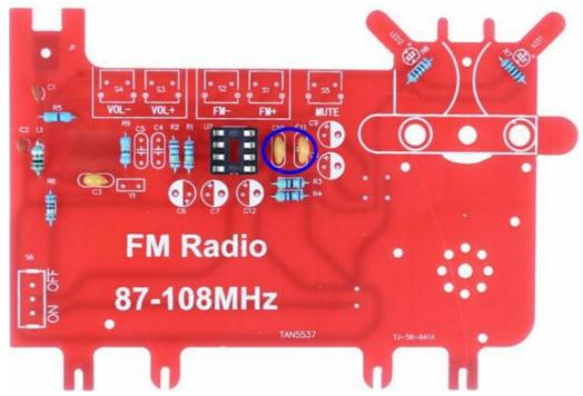
• Step 16: Install 2pcs 4.7uF 475 Monolithic Capacitor at C4,C5.
