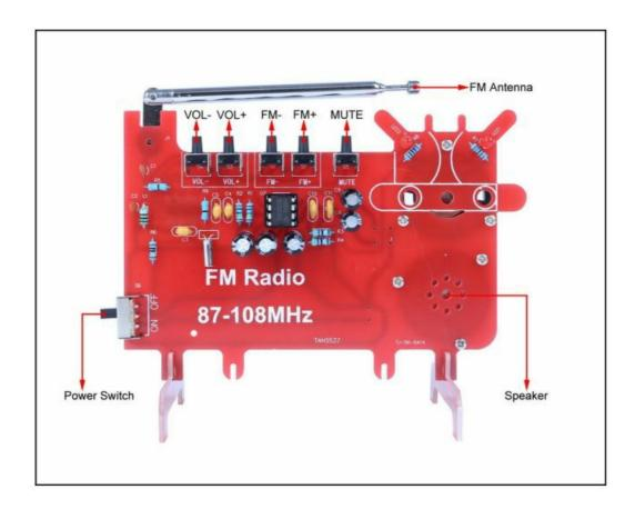
• **Step 1:** Install 1pcs SMD components SOP-16 RDA5807 FM Receiver at U1. Verify and confirm the installation direction of RDA5807. The rectangular silk screen on the PCB coincides with the crystal oscillator on the DA5807 to locate the installation direction.
