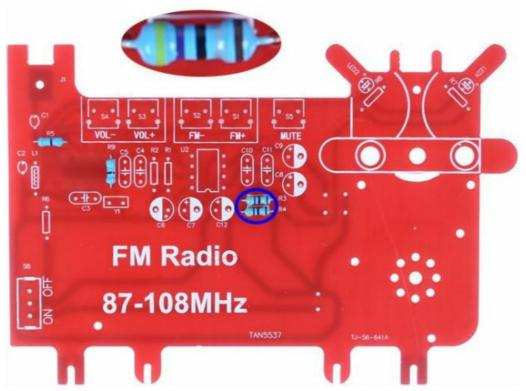
• Step 7: Install 1pcs 10ohm Metal Film Resistor at R6.
