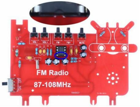
• Step 24: Install 1 pcs DIP-8 IC TDA2822 Amplifier at U2. There is a mark(notch) on one end of the IC Socket and there is a mark(curved silk screen printing) on PCB where the IC can place on. These two marks are corresponding to each other and are used to specify the installation direction of the IC.
