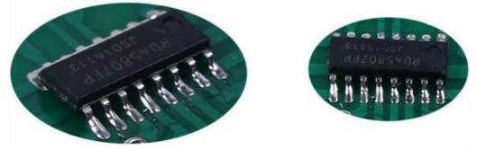
• Step 6: Check whether enough pads are filled between each pin and pad. Otherwise, you need to add more solder.
