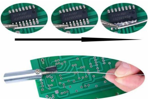
• Step 4: Melt a lot of solder on top of another row of chip pins. Make sure there is enough solder between each pin and the pad.
