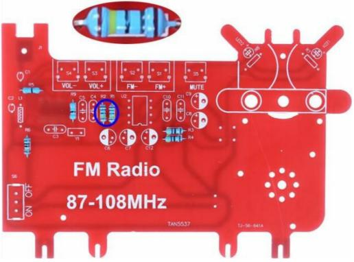
• Step 9: Install 2pcs 1 Kohm Metal Film Resistor at R7,R8.
