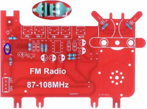
• Step 11: Install 1 pcs DIP-8 IC Socket at U2. There is a mark(notch) on one end of the IC Socket and there is a mark(curved silk screen printing) on PCB where the IC Socket an place on. These two marks are corresponding to each other and are used to specify the installation direction of the IC Socket.
