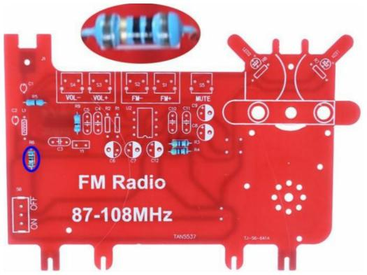
• Step 8: Install 2pcs 240ohm Metal Film Resistor at R1 ,R2.
