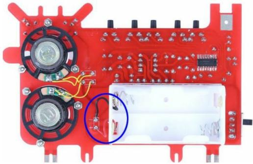
• Step 27: Fix AA\*2 battery box by its back glue and red connect to pad'+ '.
