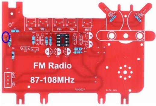
• Step 13: Install 1 pcs 1 00pF Ceramic Capacitor at C1.
