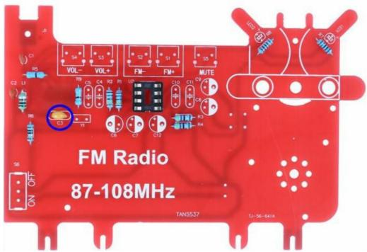
• Step 15: Install 2pcs 0.1 uF 104 Monolithic Capacitor at C10,C11.
