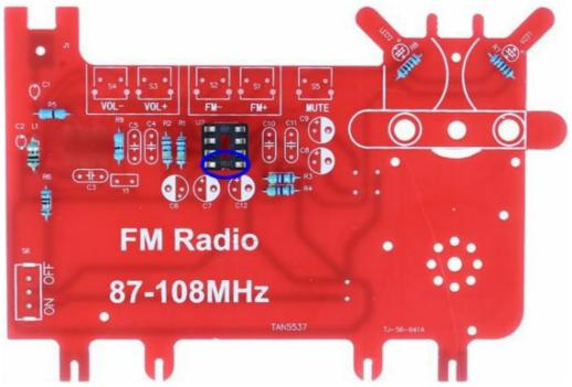
• Step 12: Install 1pcs 22pF Ceramic Capacitor at C2.
