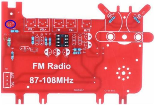
• Step 14: Install 1pcs 0.22uF 224 Monolithic Capacitor at C3.
