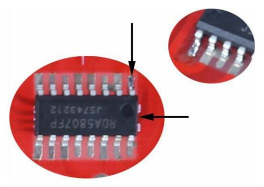
• Step 4: Connect others pads on RDA5807 to pads on PCB by tin and soldering iron.
