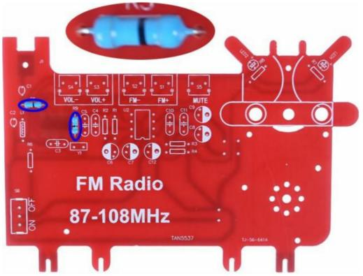
• Step 6: Install 2pcs 4.7ohm Metal Film Resistor at R3,R4.
