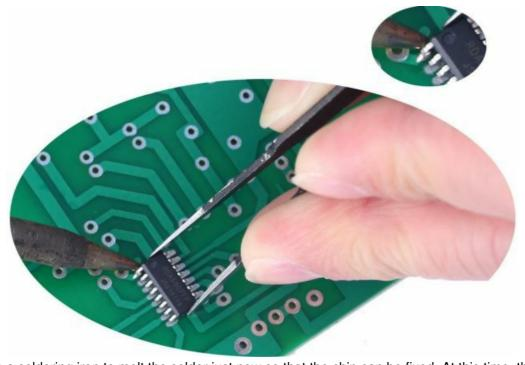
• Step 3: Use a soldering iron to melt the solder just now so that the chip can be fixed. At this time, the tweezers are still holding the chip and keep calibrating the position.
