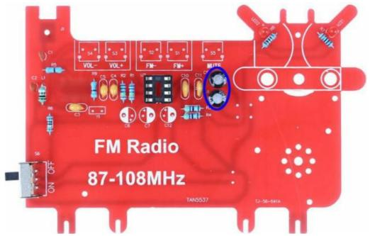
• Step 20: Install 2pcs 100uF Electrolytic Capacitor at C6,C7.
