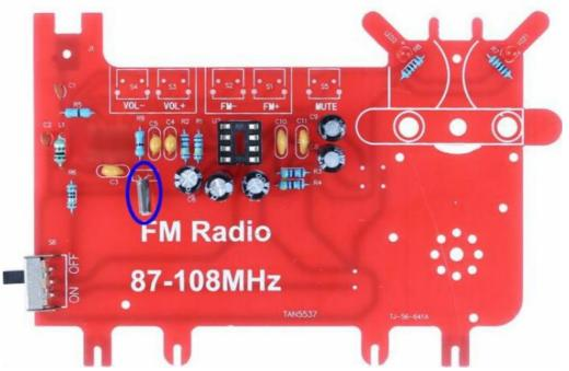
• Step 22: Install 1 pcs 32.768KHz Crystal Oscillator at Y1.
