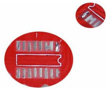
• Step 3: Fix RDA5807: Use a soldering iron to melt tin on the pad just now and hold RDA5807 with tweezers in the other hand to place/press on U1 to prevent movement. Take care to match and align each pad. Then remove the soldering iron. Then remove tweezers after solder tin cooling and solidification.
