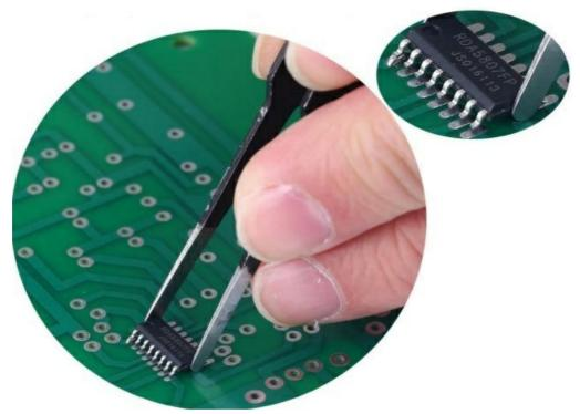
• Step 2: Hold the chip with tweezers and adjust the position so that the pins of the chip coincide with all the pads and are close to the pads.Pay attention to the mounting direction of the chip.
