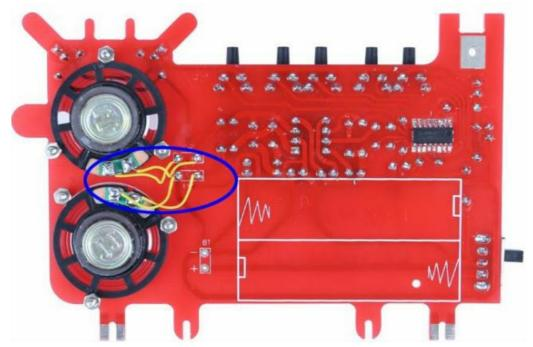
• Step 26: Connect speaker to PCB by yellow wires which can cut from 10cm wire.
