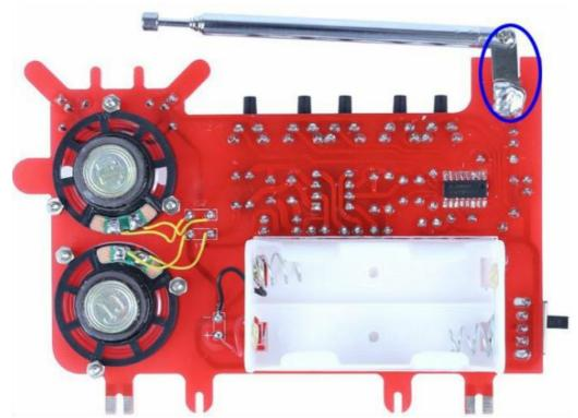
• Step 28: Install 1 pcs 75ohm Antenna at J1. Keep a distance more than 5mm from PCB and fix by tin(not screw). Note that the antenna should be installed on the back of PCB.
