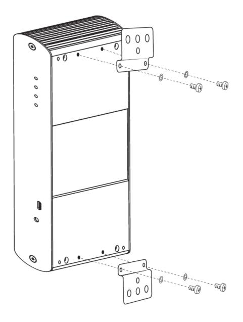
Once the bracket mounting is secured onto the extender, it is ready for mounting onto a surface. Please note you will need to provide your own screws to secure the extender using the available slots on each bracket.
