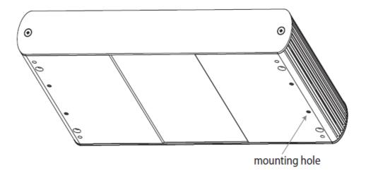
Distance between the enclosure mounting holes: 42.0mm x 205.5mm
