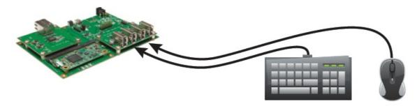
5. Connect the USB Type B port on the local extender evaluation board into a USB port on the host computer using the included USB A to B cable.
