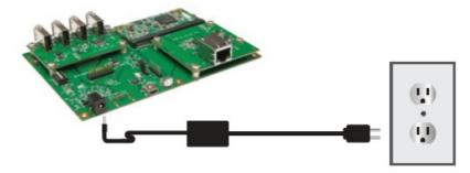
4. Connect your USB device(s) into the USB A port(s) on the USB hub module mounted on the remote extender board.
