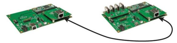
3. Connect the remote extender evaluation board to the supplied power supply and power cable, and plug it into a power outlet.
