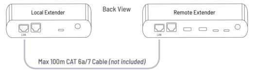
2. Power the Local Extender with the included 24V 1A AC adaptor and tighten the locking ring.
