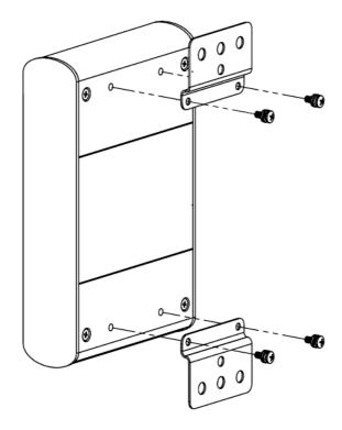
Once both mounting brackets are secured onto the extender, it is ready for mounting onto a surface. **NOTE**: You will need to provide your own screws to secure the extender onto the desired surface using the available slots on each bracket.
