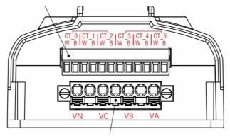
**Voltage input connector:** The pins VA/ VB/ VC/ VN are for the phase R/S/T/N of 3-phase power separately. Because the pins VA and VB are also for the working power, the iWSN-9603 series module can work normally only if the voltage between VA and VB is in the range of 100VAC – 480VAC.
