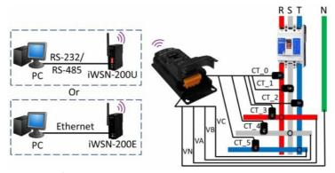
Turn ON the iWSN-200U/E and iWSN-9603 series modules to start the data collection. The RF\_Rx LED of the iWSN-200U/E flashing once indicates the iWSN-200U/E has received one message from the iWSN-9603 series module. • The flash of RF\_Rx LED indicates the iWSN-200U/E gets the data from the iWSN-9603 series module
