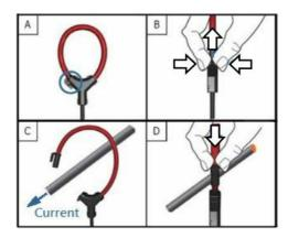
Besides the CT specification, the accuracy of Rogowski CT also depends on the location of the measured AC cable. Users must avoid putting the measured AC cable into zone D so that a smaller measurement error can be obtained.
