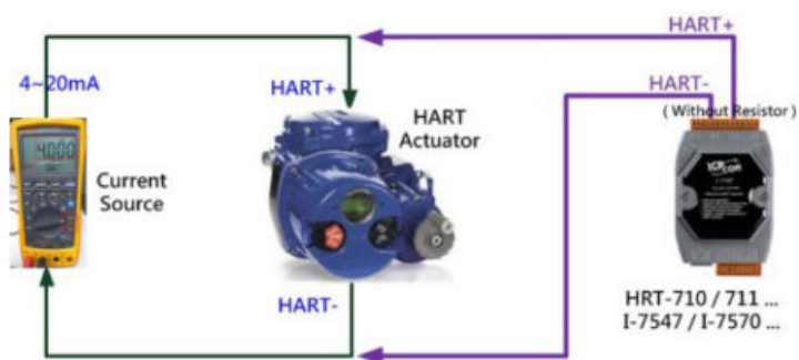
Fig 13-3-1 : "Point to Point" Mode (HART Actuator, without resistor)
