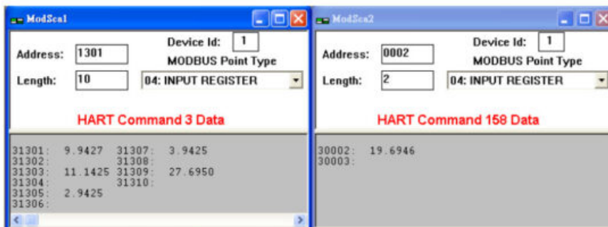
Fig 27-5 HART command 3 and 158 data shown in Modscan
