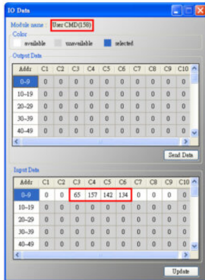
Fig 26-3 The response data of HART command 158
