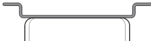
Top view of mounting bracket. Pay attention to installation direction
