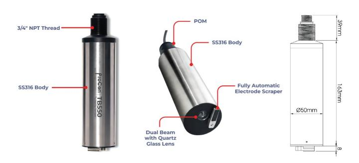
The turbidity sensor is based on infrared scattered light technology .The infrared light emitted by the light source will be scattered when it passes through the sample under test during transmission. The intensity of the scattered light is directly proportional to the turbidity.
