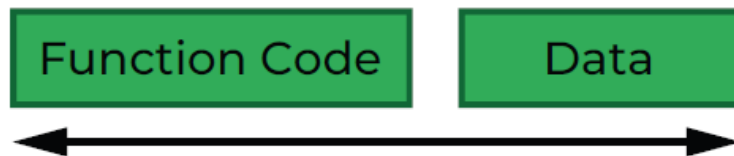
Fig.1 : MODBUS Protocol Data Unit
