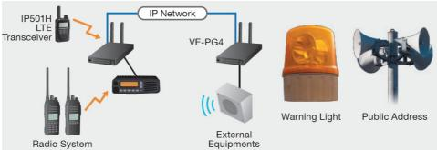
Public address system, siren, warning light and other external devices can be connected to the VE-PG4. When detecting an emergency signal, users can start emergency notification from either a digital transceiver, IP transceiver or public address system.
