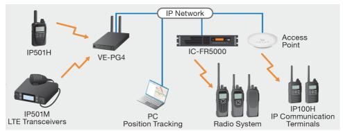
By installing a custom SIM card to the built-in LTE module, the VE-PG4 can interconnect IP501H/IP501M LTE transceivers with conventional radio systems and IP100H IP communication terminals. GPS position information from the LTE transceivers can be received and transferred to a PC.
