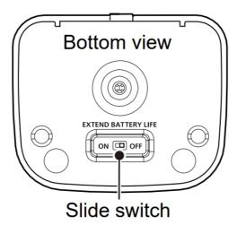
OFF: The battery is fully charged. The operating time of the transceiver is maximum.
