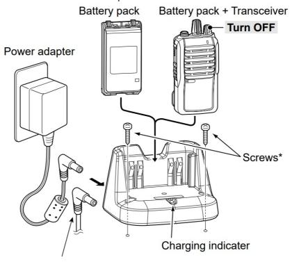
The optional OPC-515L (for a DC power source) or CP-23L (for a 12 V cigarette lighter socket) can be used instead of the power adapter.
