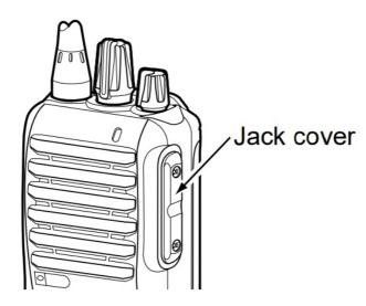
**CAUTION: DO NOT** use the transceiver without the jack cover or the optional equipment attached. The transceiver meets IP54 requirements for dust protection and splashes resistance only when the battery pack and jack cover are attached.
