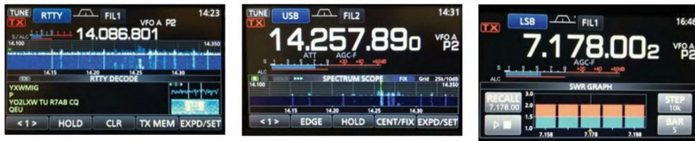
Figure 5 —The built-in RTTY decoder features a window on the lower right with a visual tuning aid — just line up the mark and space signals with the vertical bars. Up to our lines of decoded text are displayed at the lower left. You can change the bandwidths of each one, as well as the shape between "sharp" and "soft." When operating CW, it was a pleasure to select a sharp 250 Hz filter and just slowly tune through crowded bands, listening to individual signals without a hint of ringing.
