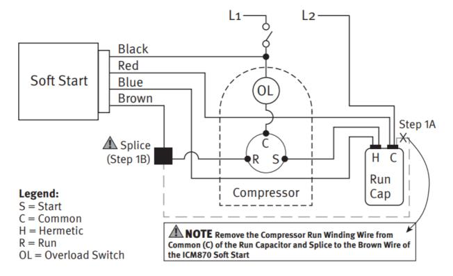
Special attention should be made concerning the termination of the field wiring leads, only at terminals suitable for a 90°C wire at minimum.
