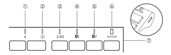
1. Charging Indicator: stay in red when charging and turn green after fully charged (about 2 hours fully charged).
