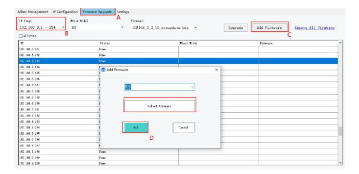
Select "Miner Model", and "Firmware", and click "Upgrade". A prompt will appear indicating the number of miners to be upgraded. Confirm the quantity and click "OK". The upgrade process takes approximately 2 minutes (Note: Do not power off during the upgrade process).
