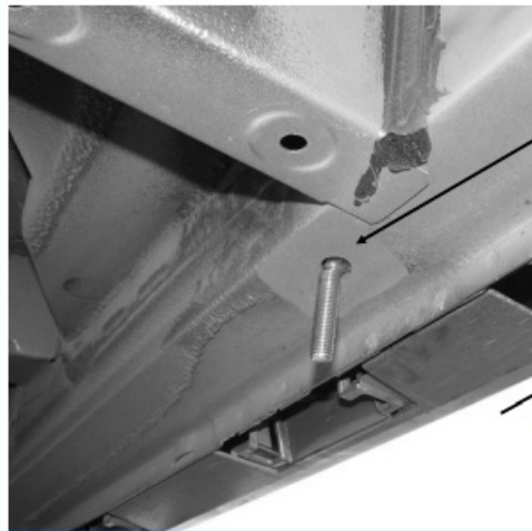
(Fig 17) Insert M10 J-Bolt With Plastic Washer Into The Hole
