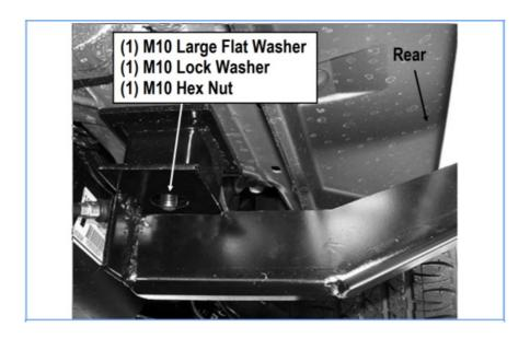
Once all (2) Driver side mounting brackets are installed, then proceed to the Step Bar installation. (Figs 6 & 7)
