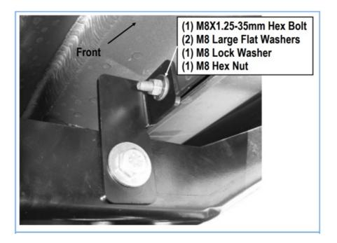
Level and adjust the Step Bar and fully tighten all hardware.
