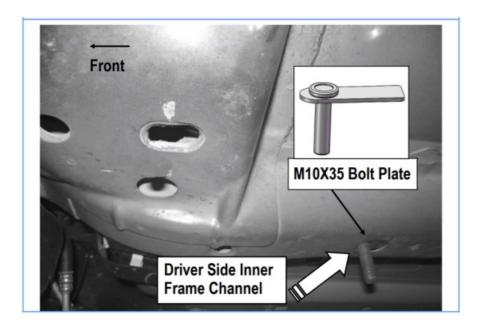
Select the Driver Front Mounting Bracket (DFM) ,attach it to the installed M10X35 Bolt Plate with (1) M10 Large Flat Washer, (1) M10 Lock Washer and () M10 Hex Nut, (Fig 2). Do not fully tighten hardware at this time.
