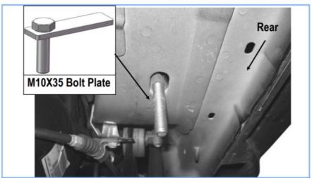
• (Fig 5) Driver Rear Mounting Bracket Installation
