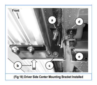
Level and adjust the Step Bar and fully tighten all hardware.
