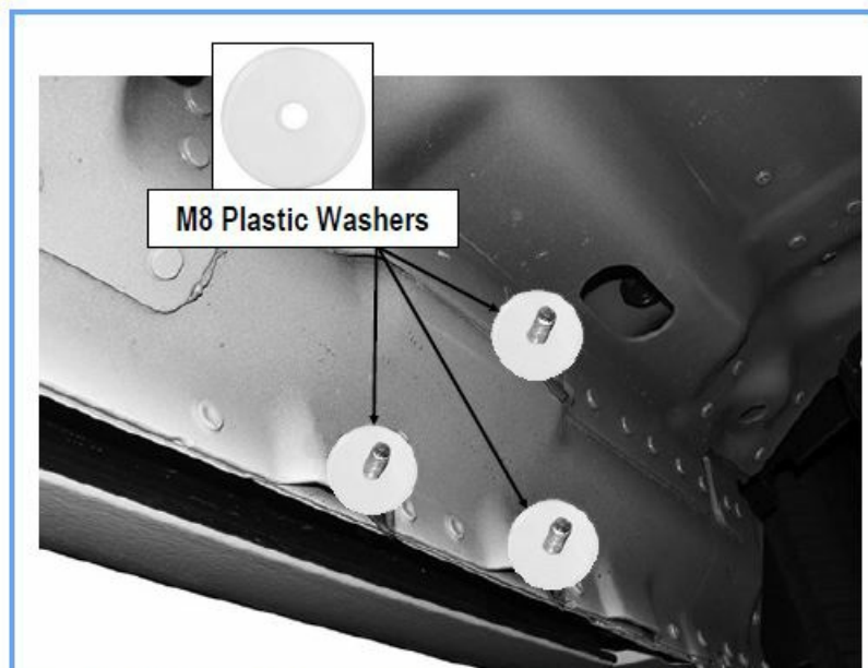
(Fig 5) M8 Plastic Washers Installed on Factory Mounting Studs
