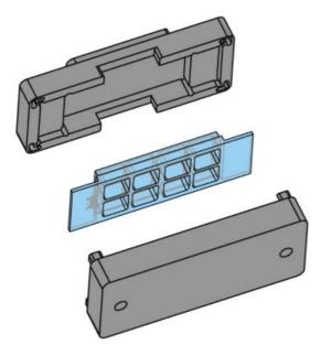
4. Mount the adapter onto the upper bracket of the clamp.
