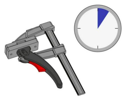
8. Open the clamp by pressing the red button and releasing the lever.
