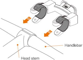
Position clamp on middle of handlebars (around any E-bike display (monitor), facing front, button-side up (rubber shims should be flush with clamp arms and sit flat on handlebars).
