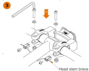
Place washers over bolt holes in clamps. Insert brace block, large hole first. Align with bolt hole, insert large bolts — ensure clamp is horizontal. Tighten well with 4 mm Allen key. Thread brace wire through one of the small brace block side holes, under head stem, then through the second hole. With wire centered, pull it taut, then fasten small Allen bolts with 3 mm Allen key.
