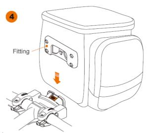
Align fitting on rear of bag with clamp mount.
