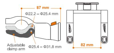
**Adjust Clamp Size.** Clamp arms have two sets of matching pin holes for smaller or larger diameter handlebars – default position suits most bars. To change setting, push pins out with 3 mm Allen key. Reinsert pin into lower holes.
