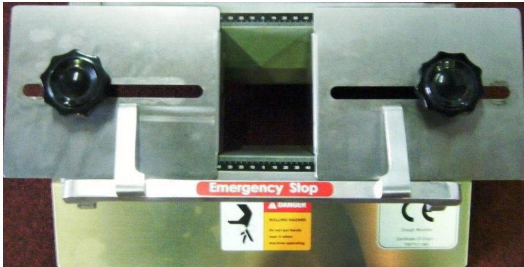
Fig1.3 In feed chute showing Emergency Stop Bar.
