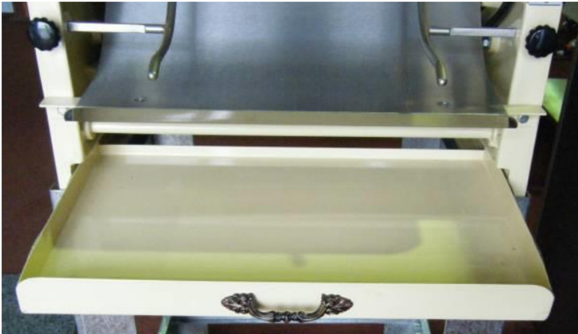
Fig1.3 Bread crumb draw, pulled out.
