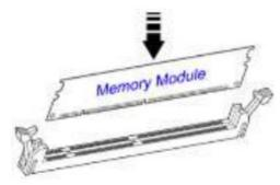
To remove the module, press the ejector tabs outwards with your fingertips to eject the module.
