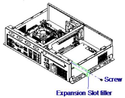
3. Install your PCIe (x16) expansion card and fix the card by tightening the screw mentioned above.
