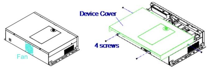
2. Remove the 4 screws shown below for fan replacement and tighten the screws after fan installation.
