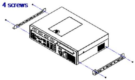
2. Prepare another four screws (M3, 6 mm) to mount the device on the target
