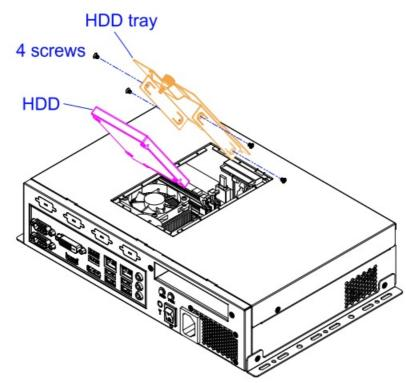
3. Return the tray back to its original position and tighten it with the screw.
