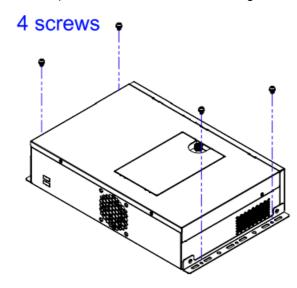
You can install CMI211 System on plastic (LCD monitor), wood, drywall surface over studs, or a solid concrete or metal plane directly. The types of fasteners required are dependent on the type of wall construction.
