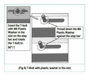
Attach the Assembled Driver Side Step Bar onto the Mounting Brackets with (6) M8 Plastic Washers, (6) M8X1.25-20mm TBolts, (6) M8 Large Flat Washers, (6) M8 Nylon Lock Nuts, (Fig Do not fully tighten hardware at this time.
