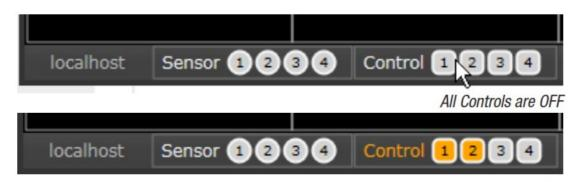
Controls 1,2 are ON; Controls 3,4 are OFF.
