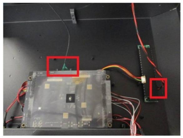
Step 4: Remove these 4 screws to release the AD board.
