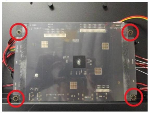
Step 5: Flip over the AD board and disconnect all the connected wires, and then replace with new AD board.
