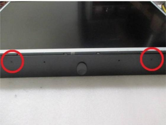
**Step 3:** Lift up the panel and disconnect the LVDS & inverter wire slowly and carefully for prevent the damage to both panel & wire, and remove the panel set out of its chassis.
