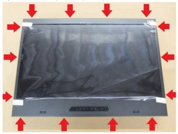
**Step 2:** Remove the LCD mounting screws (8 screws, 3 on each side, 2 on top).
