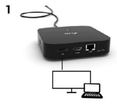
1 monitor connected via 1x DP cable – resolution up to 5K 5120×2880/60Hz. 5K resolution is only supported if your laptop's USB-C/Thunderbolt™ 3 connector supports DisplayPort 1.4 DSC.
