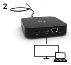
1 monitor connected via DisplayPort/HDMI cable – resolution up to 4K 3840×2160/60Hz. 4K/60Hz resolution is only supported if your laptop's USB-C/ Thunderbolt™ 3 connector supports DisplayPort 1.4 DSC or DisplayPort 1.4 without DSC. If the USB-C/Thunderbolt™ 3 only supports DisplayPort 1.2, the maximum resolution is 4K 3840×2160/30Hz.
