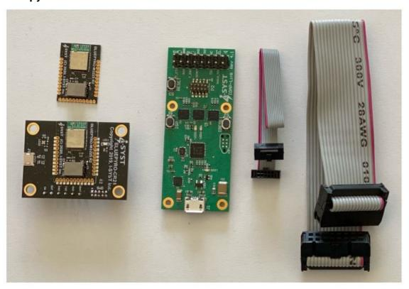
Prepare Bluepyro-M3225 development kit as the figure above include Bluepyro-M3225 board, IDAP-Link. Connect Bluepyro-M3225 to computer.
