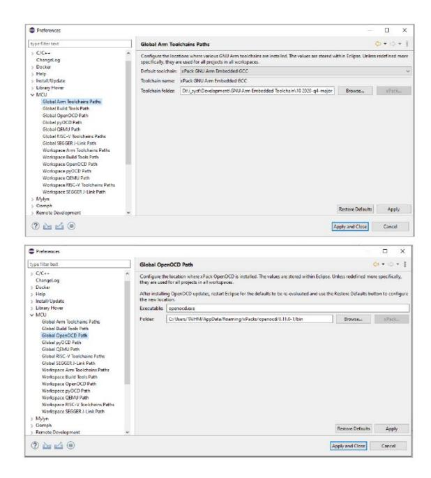
That is all that's needed for Eclipse and toolchain installations. This Eclipse installation is not limited to Nordic based development. It is a generic installation that allows you to work with any ARM Cortex MCU from any vendor. It works for RISC-V as well. You will need to install toolchains for RISC-V if you want to work with that in Eclipse.
