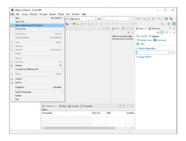
A pop-up will open. Click on the "Directory" button, navigate to, and select the 'nRF52832' folder in the IOsanota/ARM/Nordic/nRF52/ location. Eclipse will search and list all projects available within that folder. Deselect the first checkbox 'nRF52832' and keep all the others. For the BLYST840, use the 'nRF52840' instead.
