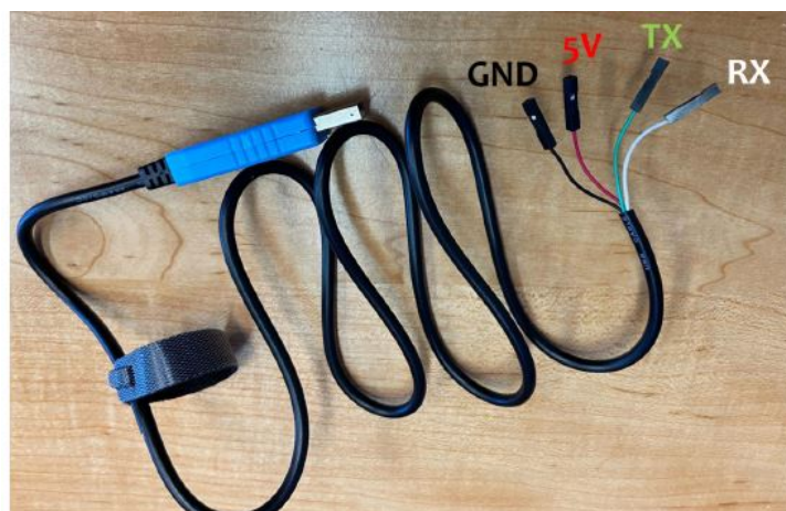
Fig. 5. UART's pins on USB-UART adapter. UART-TX (Green), UART-RX (White), 5V power supply (Red), and Ground (Black)
