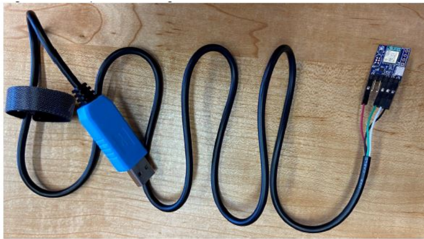
Fig. 6. Connect BlueIO832-Mini with a USB-UART adapter. The 5V and GND cables can be used for powering BlueIO832-Mini thanks to its internal level shifter.
