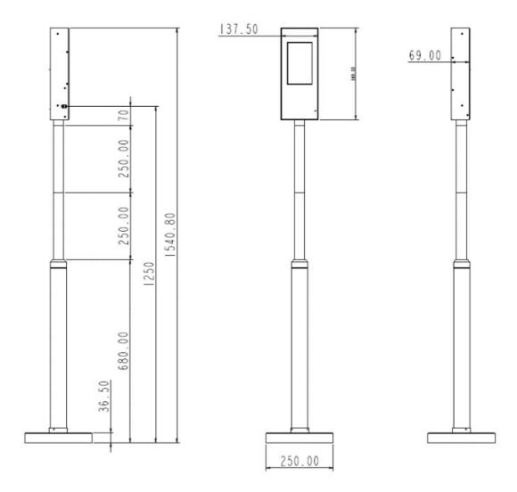
The figure below shows the structure and cable of the device. The actual device may vary.
