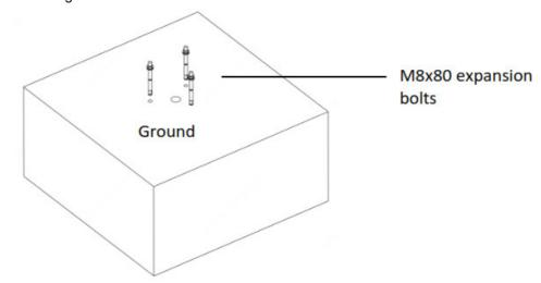
6. Erect the standing pole, align the hole position at pole bottom with the expansion bolts fixed on the ground, adjust the standing pole so that it's perpendicular to the ground, adjust device direction, and then fasten the standing pole with nuts.
