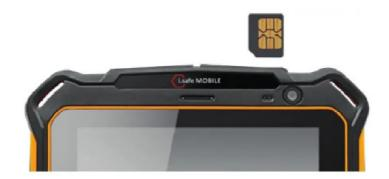
**WARNING** Do only change the SIM card when the device is switched off. Do not try to insert or remove the SIM cards when any external power supply is connected, otherwise, the SIM card may be damaged.
