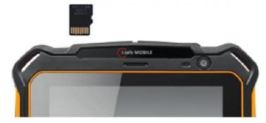
**WARNING** Do only change the microSD card when the device is switched off. Do not try to insert or remove the microSD card when any external power supply is connected, otherwise, the microSD card may be damaged.
