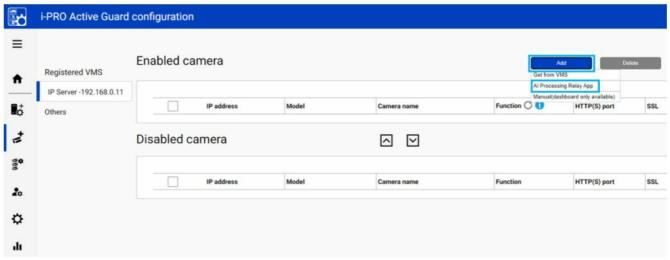
3. Enter the IP address and authentication information for the new X series camera, and click "Check". Confirm that the non-Al camera appears in the list and click "Save".
