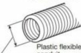
Plastic flexible conduit Inside diameter ø14 mm {ø9/16 inches}
