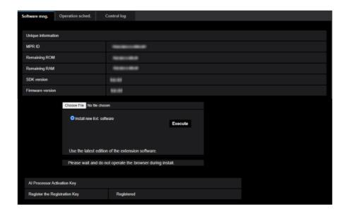
When the extension software is installed, unique information of the camera and the registration status of the extension software will be displayed. On this screen, the following operations are available.
